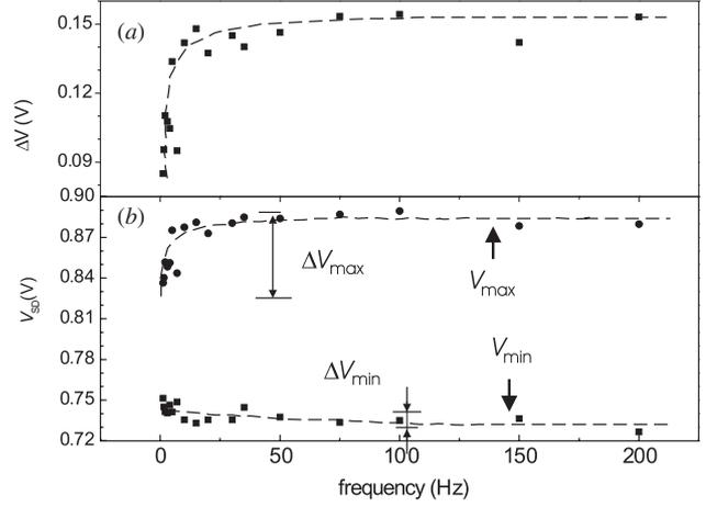
**Figure 3.** (a) The frequency dependence of the amplitude of the QH breakdown hysteresis, (b) the frequency dependence of the limits of the hysteresis curve,  $V_{\min}$  and  $V_{\max}$  of the Corbino sample with a channel width of  $100 \mu\text{m}$ .
