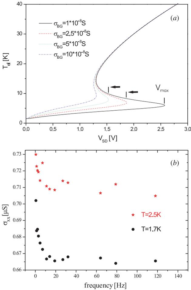
**Figure 4.** (a) Calculated electron temperature  $T_{el}$  versus  $V_{SD}$  for different background conductivities  $\sigma_{BG}$  for a sample channel width of  $200 \mu\text{m}$ . (b) Frequency dependence of the background conductivity in the pre-breakdown regime at a constant voltage (0.8 V) for two temperatures (1.7 K and 2.5 K).
