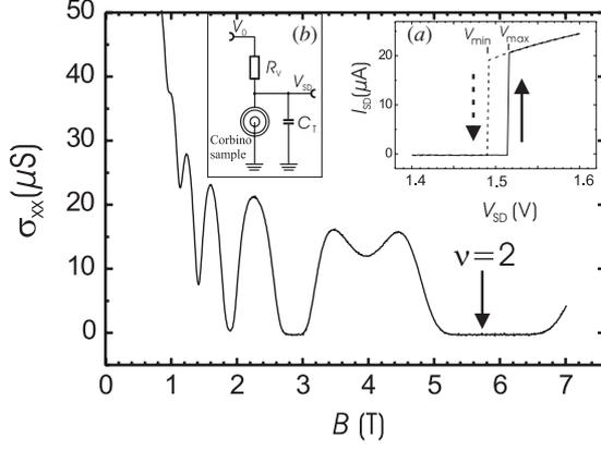
**Figure 1.** Shubnikov–de Haas oscillations (at  $V_{SD} = 100$  mV) of the QH–Corbino devices. Inset: (a) dc current–voltage characteristics of the Corbino sample with a channel width of  $200 \mu\text{m}$  at  $B = 5.7$  T (second QH plateau,  $T = 1.5$  K). (b) Scheme of the oscillator circuit:  $V_0$ : driving voltage,  $R_V$ : serial resistor,  $C_T$ : total capacitance.
