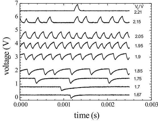
**Figure 2.** Relaxation oscillations of the Corbino device at different driving voltages  $V_0$  (curves shifted for clarity).  $R_{CB} = 90$  k $\Omega$ ,  $R_V = 46$  k $\Omega$ ,  $C_T = 1.5$  nF.
